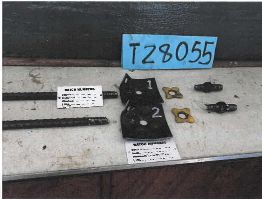
Figure 2. Roof bolt assemblies (20 mm x 1.5 m) after testing
