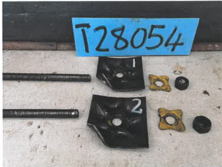
Figure 2. Roof bolt assemblies (18 mm x 1.5 m) after testing
