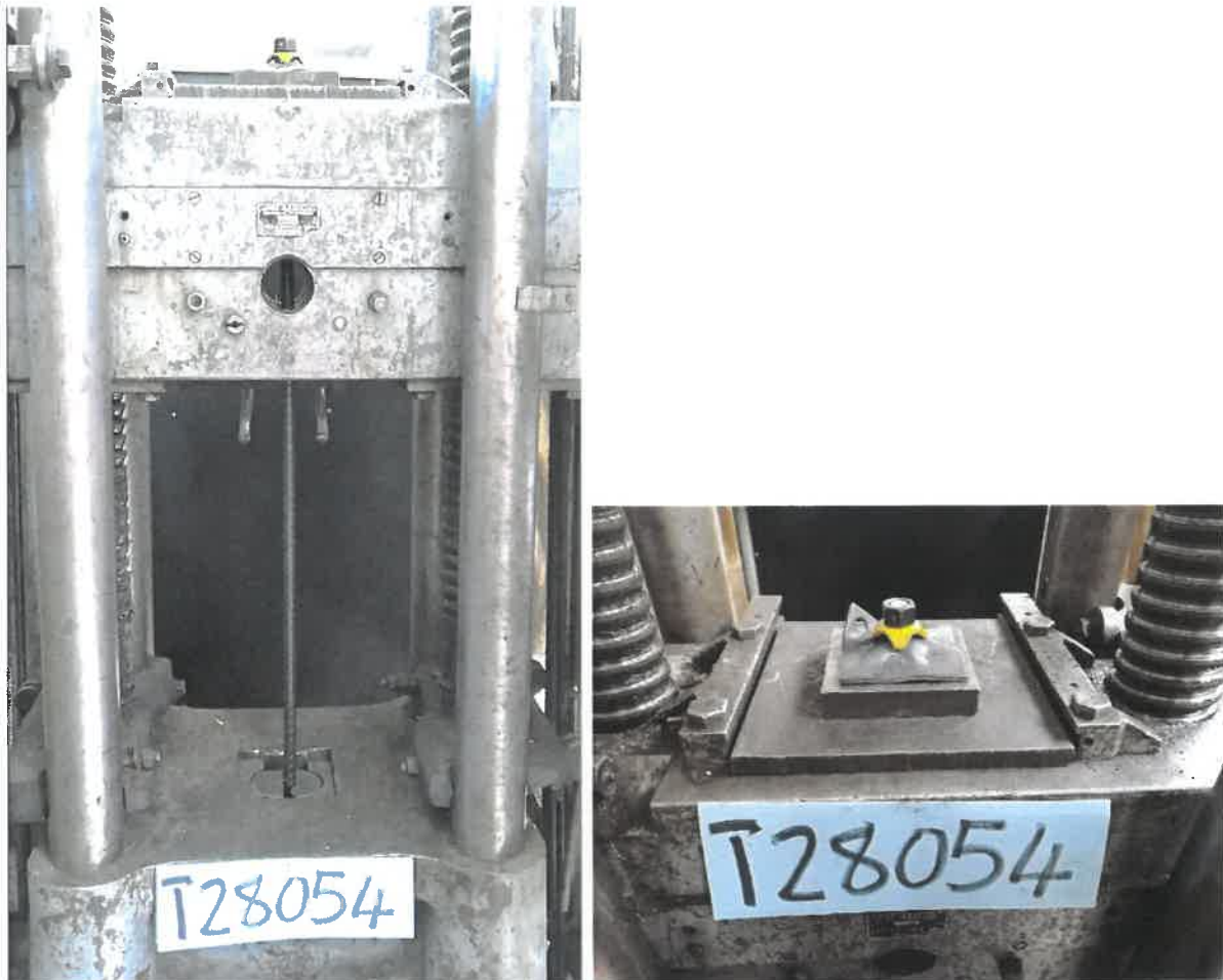
Figure 1. Roof bolt assembly (18 mm x 1.5 m) installed in the testing machine
