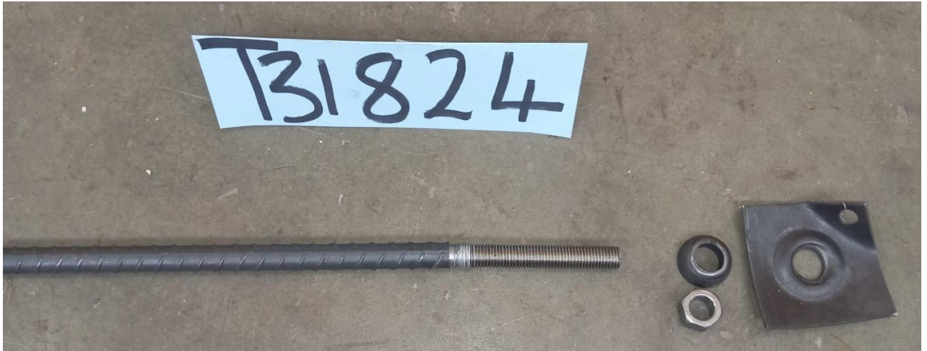
Figure 2. Roof bolt (MB25 mm x 1.0 m) after the test.
