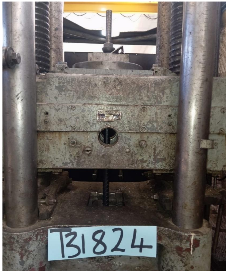
Figure 1. Roof bolt (MB25 mm x 1.0 m) installed in the testing machine.
