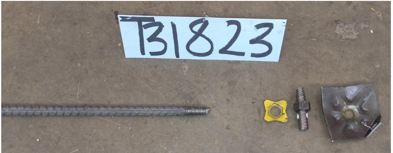
Figure 2. Roof bolt (MB20 mm x 1.8 m) after the test.
