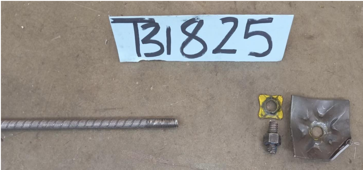
Figure 2. Roof bolt (MB18 mm x 1.2 m) after the test.
