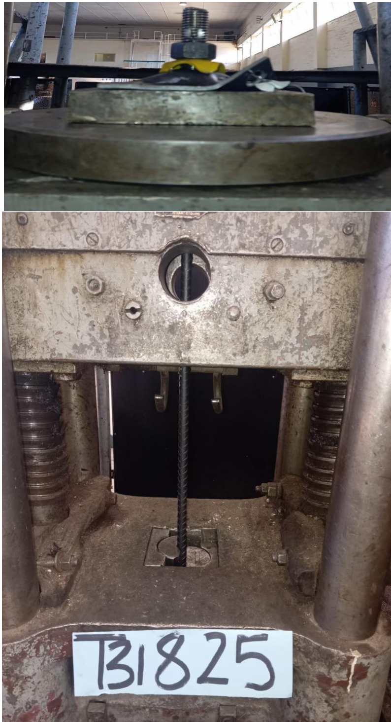
Figure 1. Roof bolt (MB18 mm x 1.2 m) installed in the testing machine.
