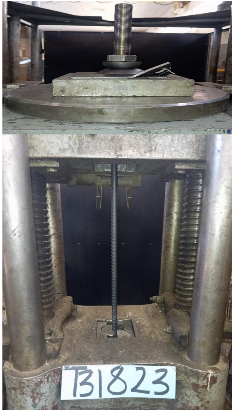
Figure 1. Roof bolt (MB20 mm x1.8 m) installed in the testing machine.
